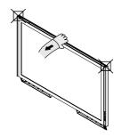
Hold onto the middle of the PDP to adjust the angle (not the sides of the PDP).
